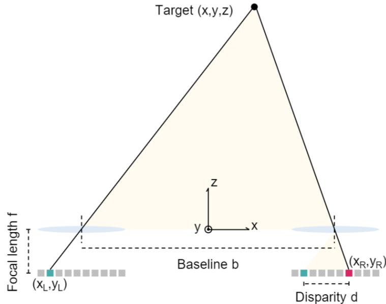
Schematic of binocular stereo vision
